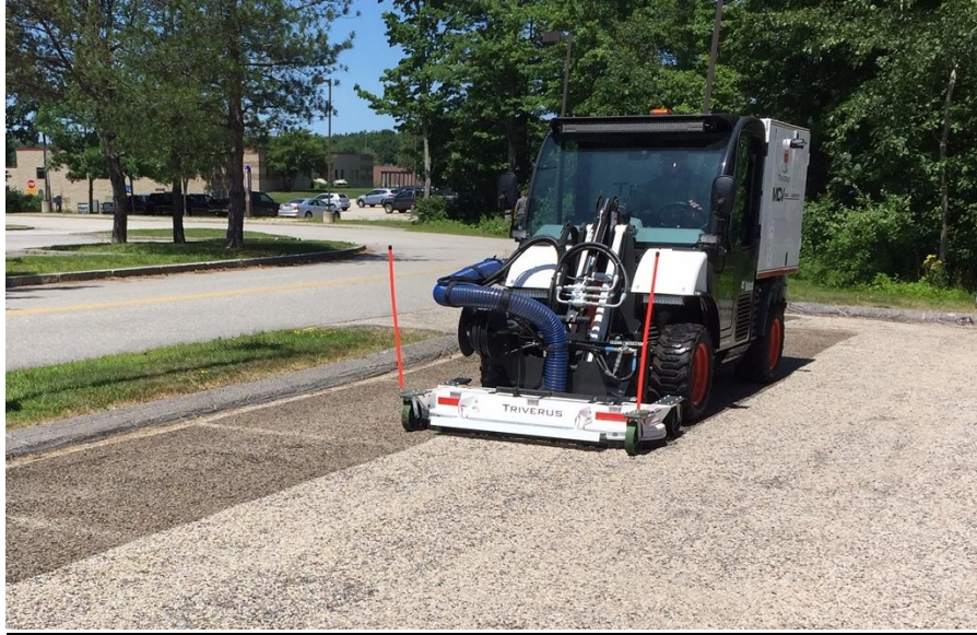
Figure 1: Triverus MCV cleaning West Edge Porous Asphalt (UNHSC).
