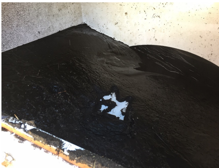
Figure 8: The fines collected in the collection tank after coarse solids were removed in the tray screen and the water was pumped out. Note the center where the fines were moved to show the bottom of the tank (white).
