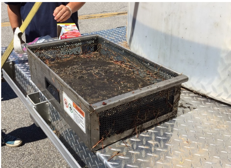
Figure 7: The coarse solids collected in the solids tray after several passes on the West Edge PA.
