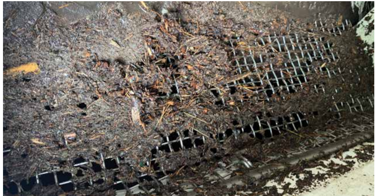
The coarse solids collected in the solids tray after several passes on the West Edge PA.
