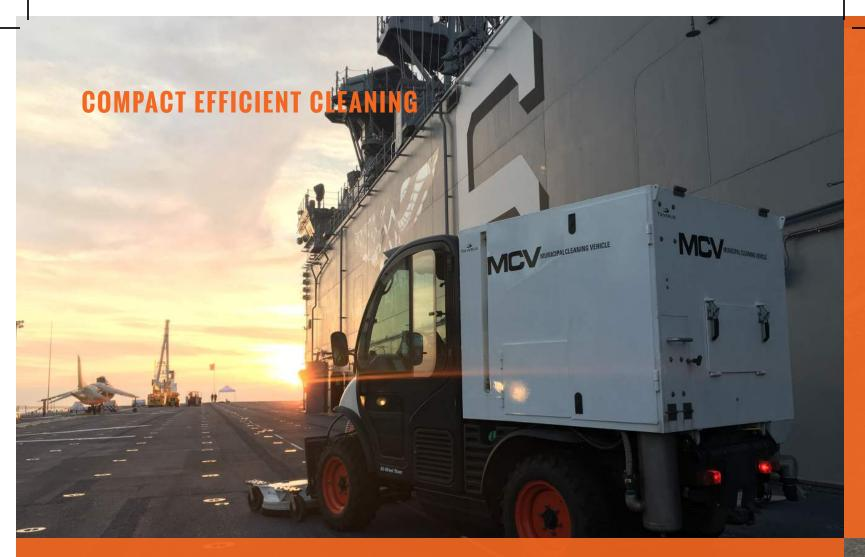
The Municipal Cleaning Vehicle (MCV) packs high efficiency cleaning capacity into a compact and versatile standards-based platform. The 5 ft wide cleaning path provides for excellent productivity while still performing tasks inside parking facilities, sidewalks and other spaces where size and maneuverability count.
